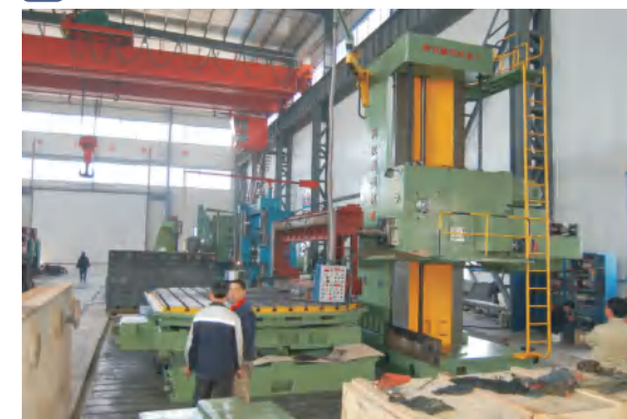
↑ 200mm数控落地镗床 200mm electric control floor-type boring and milling machine
