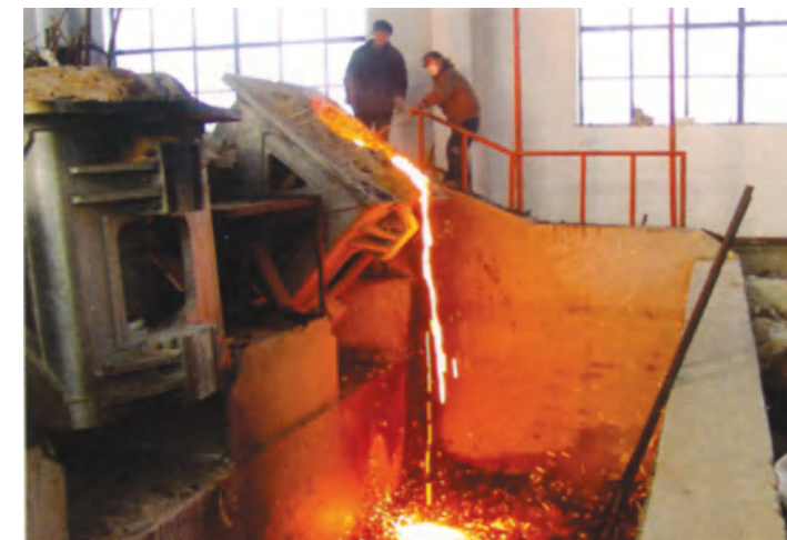
↑ 10吨中频炉 10t Mid-frequency electric oven
