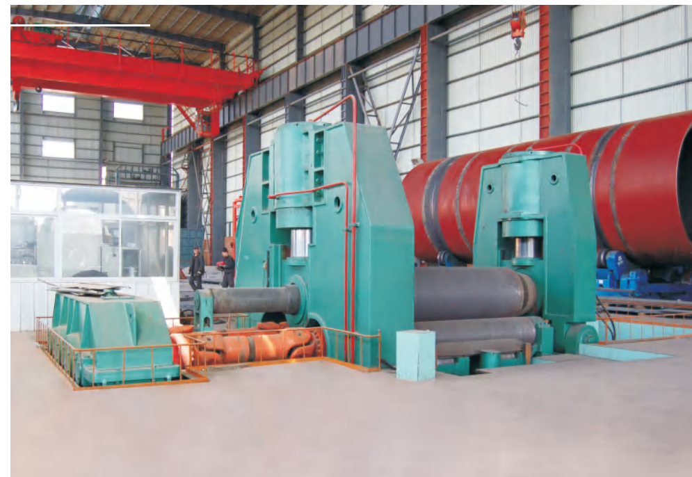
↑ 120×3200卷板机 120×3200mm three-roller plate rolling machine
