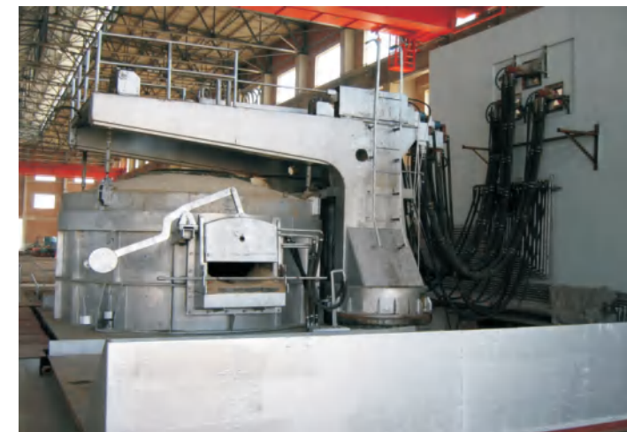
↑ 40吨CPU自动控制电弧炉 40t electric furnace controlled by national improved CPU automatically
